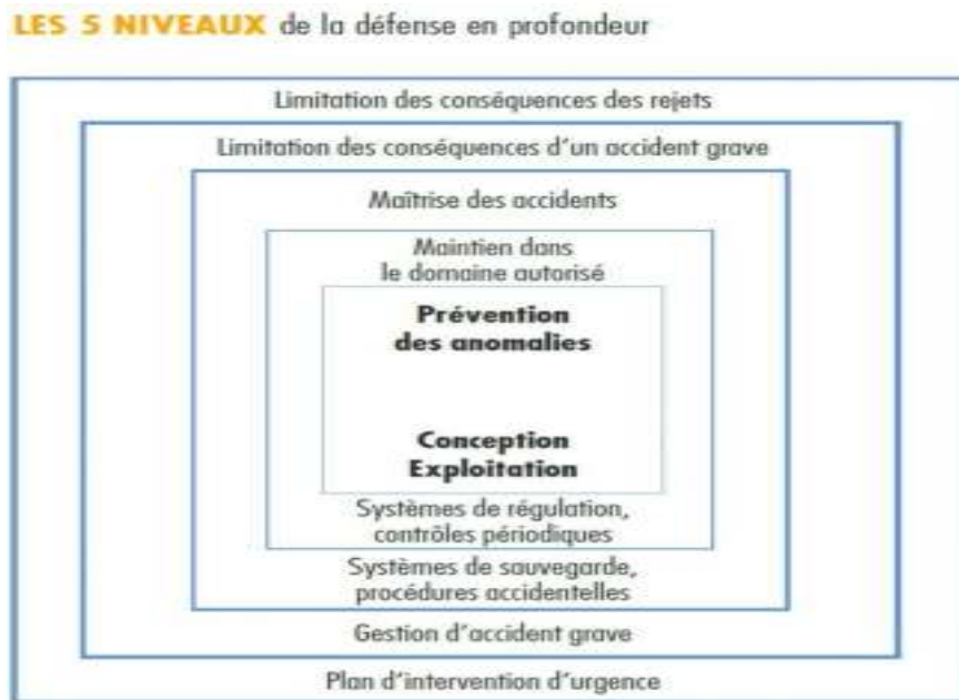
Figure 32: The nuclear safety principle "defence in depth"
